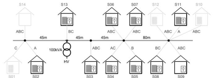
Figure 1. Electrical connection diagram of field trial site
