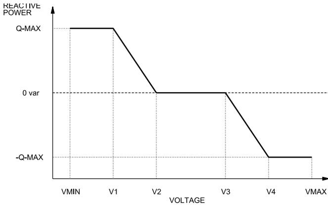
Figure 2. Statcom volt-var response curve.
