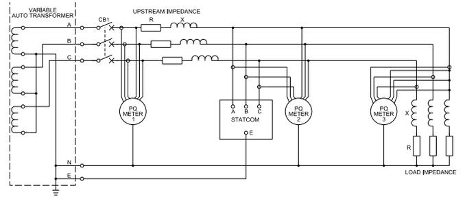
Figure 3. Electrical connection of laboratory test.
