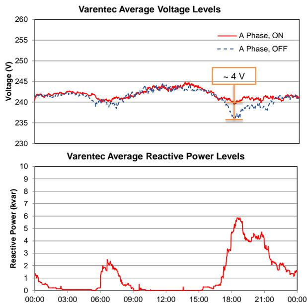
Figure 6. ENGO voltage improvement during field trial.
