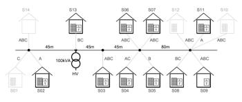
Figure 1. Electrical connection diagram of field trial site
